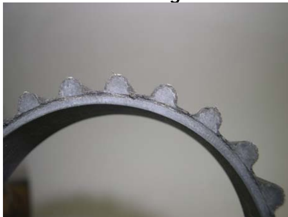
Fig. 2 Conventional timing belt
